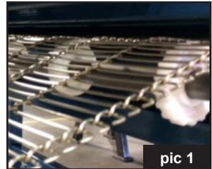
13. At the exit end, connect the two ends of the belt together with the provided belt splices. The splices are taped onto the belt's edge. An extra set is in the envelope with the belt.
