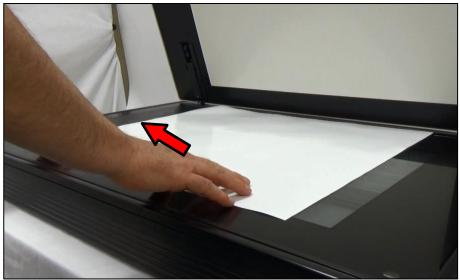
2. Correctly insert the calibration target onto the scanner with the targets arrow pointing towards the left.
