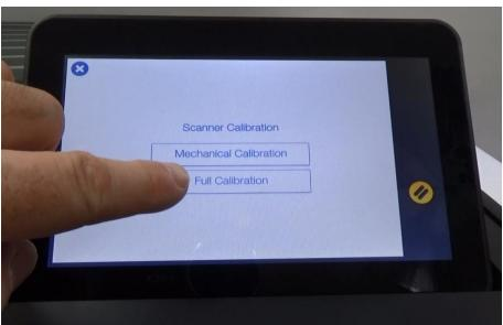
6. Click 'Full Calibration'. The Calibration will take about 27 minutes. Remove the target when completed.
