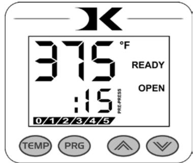
The word PREPRESS will be displayed next to the pre-press time setting when it is active. To set the pre-press time, simply use the Arrow Keys to set the time. If PREPRESS is not displayed next to the time, quickly close and then open the press to switch to the prepress time.
