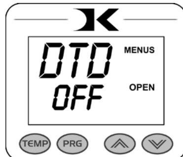
If the current temperature drops below the set temperature by that many degrees, the timer will not operate, and therefore on an automatic press, the press will not activate. The press will “unfreeze” once the temperature is within set point by the value selected or less.
