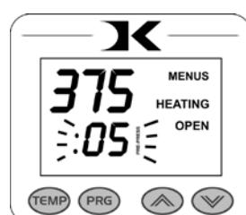
Press the TEMP key. The Pressure reference value will flash. Use the Arrow Keys to set the pressure for that preset. This will display 0 to 9 for presses configured for Bar Graph Pressure readout, and will display 0:00 to 10:00 for presses configured for a Height Gauge readout.
