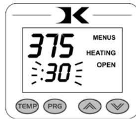
Press the TEMP key. The Prepress time will flash. Use the Arrow Keys to set the Prepress time. Set the Prepress time to 00 if only one timer is to be used for that preset. [Setting Prepress to 00 will disable the Prepress feature.](#)
