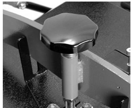
**WARNING:** The heat platen will become detached from the frame and drop onto the table if it is adjusted too far.
