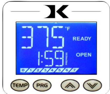
The right side of the screen will also indicate the timing status by stating OPEN, TIMING or DONE. The DONE indicator may remain on in some cases until the press is opened back up.
