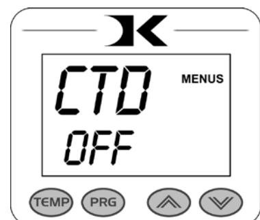
When this feature is ON - the normal countdown timer display is replaced by this odometer instead. The arrow keys no longer adjust the countdown timer, but instead are used to set the countdown odometer. When OFF, the timers are visible.
