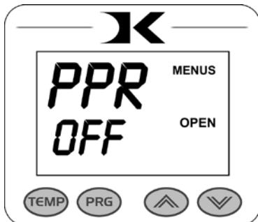
After entering the user menus (see top of page 14), Press PRG until PPR displays. Use the arrow keys to set it to ON or OFF.
