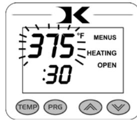
Press the TEMP key. The time will flash. Use the Arrow Keys to set the time for that preset.
