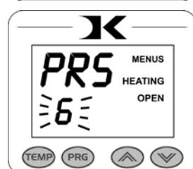
Press the TEMP key. The screen returns to the preset #. Press PRG to return to the normal operating mode, or use the Arrow Keys to select a different preset and edit that as well.
