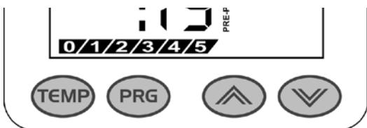
If the pressure adjustment has been changed, or a different thickness item has been placed in the press, the pressure bar graph will not change until the press is closed and locked and the timer is counting.
