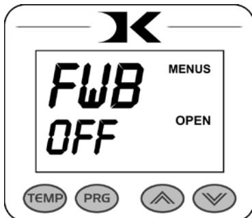
After entering the user menus (see top of page 14), Press PRG until FWB displays. Use the arrow keys to set it to ON or OFF.
