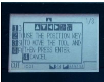
You'll now need to do a test cut. Press the **RIGHT Arrow** button on the front panel to be taken to a screen that lets you use the **Arrow** buttons to move the cutter blade to a position on the paper you'd like to cut.
