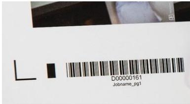
On every Cut-it-out! enabled print, a barcode is generated (along with the job name and the job number that appears for the job in Spoolface). For the Graphtec CE-6000 and FC-8600 the bar code should be loaded **first** into the cutter. For the Lite CE-50, load the end of the paper opposite of the barcode first--the barcode goes last for that cutter.
