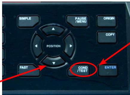
On the cutter's control panel, press the **COND/TEST** button.
