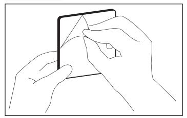
**Step 1:** Peel film off the coaster. Clean the surface of the coaster with a clean lint-free cloth, and all-purpose cleaner, or a can of compressed air. This will ensure nothing is on the surface of your product for sublimation.
