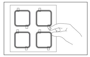
**Step 2:** Line up the coaster to the transfer. Using heat tape, secure the coaster to the transfer. With bare sides facing up, place in heat press. Time may vary based on equipment. You may need to increase time if pressing more than one coaster at a time.
