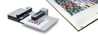
The Spectro LFP qb Digital Press edition offers fully automated reflection measurements for materials up to 20 mm with its variable 2-6 mm measurement aperture. It is made to measure paper and paperlike material and a variety of packaging materials like carton and corrugated.
